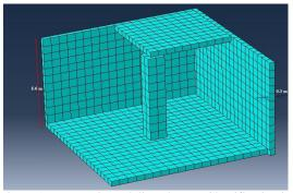
Figure 1 - Reservoir modeling element Classification in ABAQUS
