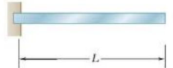
(c) Cantilever beam
