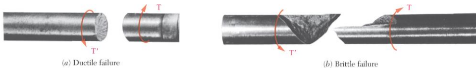
Photo 3.2 Shear failure of shaft subject to torque.
